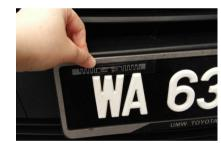
\*\* Please DO NOT place the sticker on metal surface / windscreen or near any metallic object. Metal will severely inhibit reading range.
