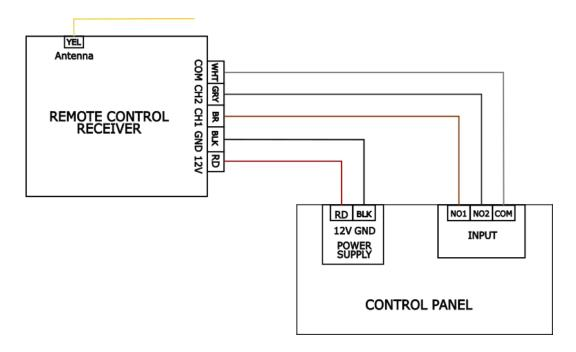
Note: It's Universal Remote that supports remote and wirelessly controls your autogate, garage door, electronic gates, electrical appliances and other telecommand equipment.
