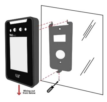
Install The Wall Bracket and device to a Glass Surface
