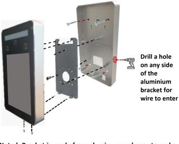
Noted: Bracket is made from aluminum and easy to make a hole for surface installation \*Wall Mount Sold Separately
